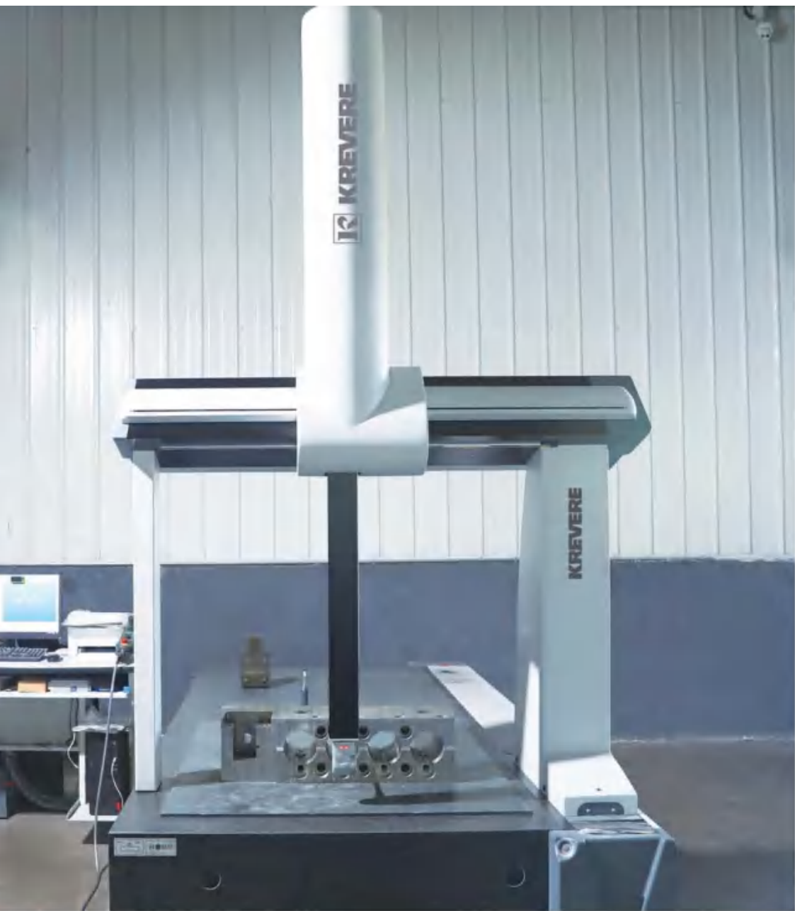
大型三坐标测量设备，确保每台出厂机器的零部件精度。 Large CMM equipment ensures the accuracy of parts of each factory machine.
